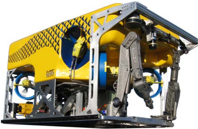
Figure 21 – Remotely Operated Vehicle (ROV) – ROV making electrical connection (courtesy of Schilling Robotics - www.ssaalliance.com )
